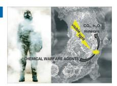
Self-decontaminating textiles were prepared using layer-by-layer deposition of highly active WO<sub>3</sub>/titanate nanotubes for photocatalytic removal of sulfide and organophosphonate simulants and authentic chemical warfare agents by using solar light.
